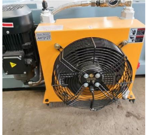
550B reducer Air cooling system
